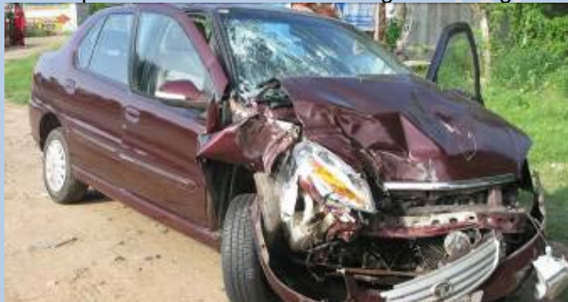
Figure 2: Frontal impact damage
