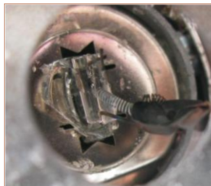
Oxidized filament with tungsten oxide on the surface
